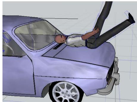
Fig. 2.2.1. Dynamics of pedestrian impact at 40 - 50 km/h
