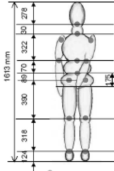
Fig. 1.3.1. Dummy model
