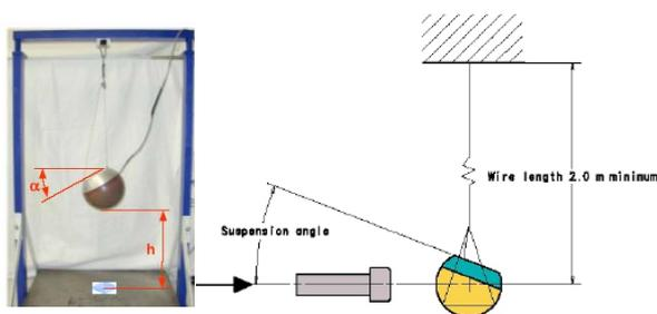
Fig. 1.2.2. Drop test and pendulum test
