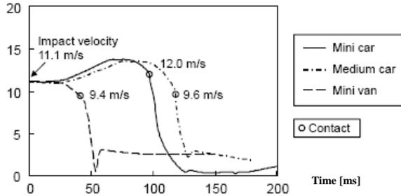
Fig. 1.4.4. resultant head velocity to the vehicle
