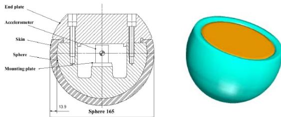
Fig. 1.2.1. Artificial head model
