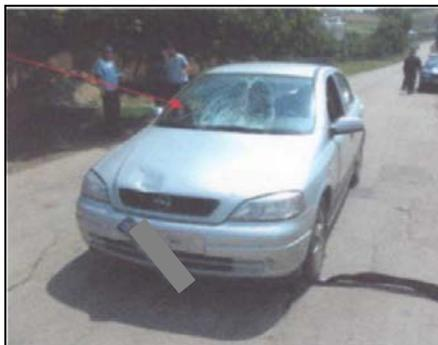
Fig.2.2.4. Impact at 68 km/h velocity with adult pedestrian and Opel Astra vehicle
