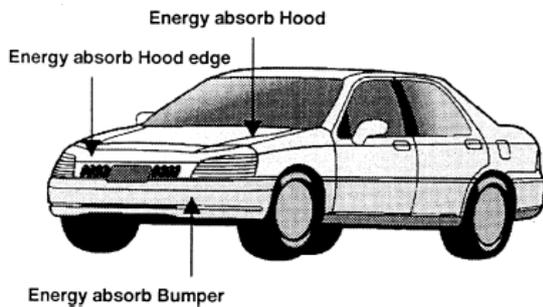
Fig. 1.4.1. Front parts of the vehicle were the most of energy is discharged
