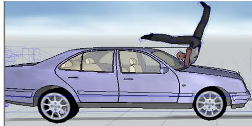
Fig.2.2.5. Dynamic impact at 60 - 80 km/h velocity with adult pedestrian
