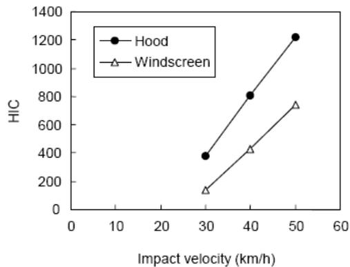
Fig. 2.1.1 Effect of impact velocity on the HIC for tested car
